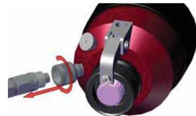
8.5 Plug the uncoupled end of Pre-Setting head with the protective plug removed and stored earlier.
