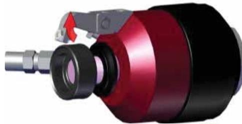
6.2 Open the release valve on the hand pump (turn counter-clockwise). Insure the end of the Die is back from the end of the threaded portion of the Jig.
